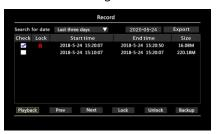
Searching by latest 3 days / one week / fortnight / a month. Video can be playback and backup from saved video files. Select needed file for backup by External USB flash drive, pull out flash drive after backup program processed. Note:
