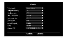
Record for park: After the flame-out, the device will continue to be in the recording state, which can be set directly Close or prolong the time to close, the delay time is 10 minutes / 30 minutes / 1 hour /1 hour /2hour /6hour /12hour/24hour: Audio recording: Recording can choose microphone or camera to collect audio, if you do not need to choose to close; Channel Titleset the channel title display, you can choose CH01.CH02.CH03.CH04 /Left.Right.Front.Back / Close three modes:
