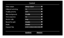
Video output: Intelligent output/always output /Trigger output Delayed switching: select time 1 sec /2sec ......./15 sec; Display priority: Set trigger single channel picture priority; Blue backgtound: Set blue screen background on / off; Auto sequence: Set CH01 / CH02 / CH03 / CH04 single channel automatic switching screen Time 1 second. 2 seconds ... 15 seconds or closed:
