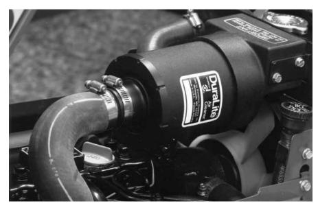
DuraLite™ Air Cleaners — sturdy, one-piece, and disposable — are designed to withstand the high pulsation of small engines such as the ones shown here. They are easy to maintain because there are no service parts. When the filter is full, simply throw it away.
